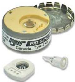
Photoionization sensor available for volatile organic compounds (VOCs) detection.
